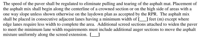
The Engineer should specify the widest paving lane practicable in an effort to hold the number of longitudinal joints to a minimum. Additional job specific construction limitations may be added as necessary covering such items as echelon paving, hot joint construction, etc.
