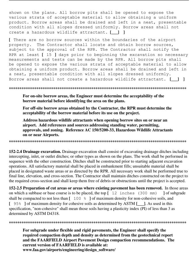
Specify ASTM D698 for areas designated for aircraft with gross weights of 60,000 pounds (27200 kg) or less and ASTM D1557 for areas designated for aircraft with gross weights greater than 60,000 pounds (27200 kg).
